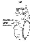
6. When the highest frequency is reached maximum power has been set. From this point, turn both adjustment screws 1/4 turn clockwise. The regulator is now set.
